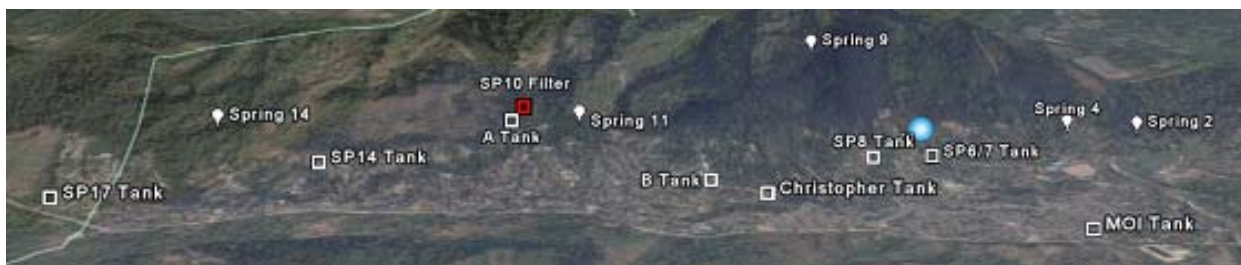
Figure 2-3: Major Water System Components.
